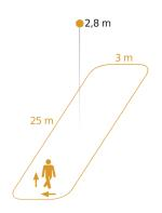
Possible mounting height: 2,50 m – 3,50 m Orange: radial and tangential
